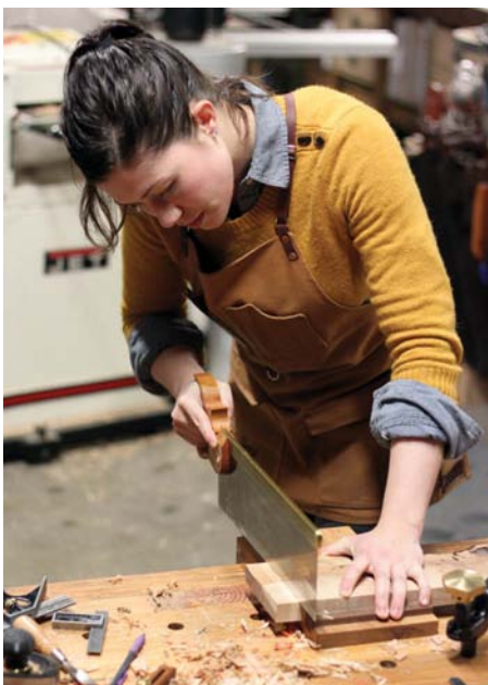
Establish the sides of the dado with the saw
