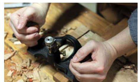
Meet in the middle to avoid blowout
