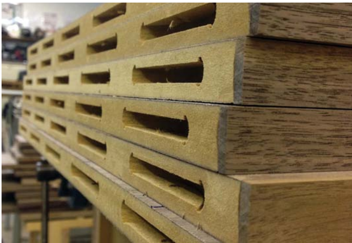
Axe head style slots for the Lamello Zeta P2
