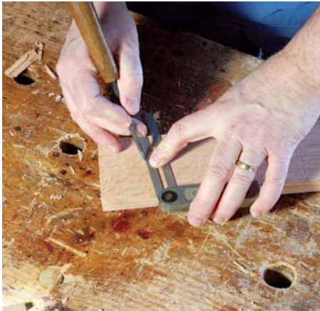
Adjustable bevellers are often small enough that you can grip the handle and blade in one hand, pinching the whole tool against the rail's top edge. However you hold the tool, be sure it has not lost its setting and keep it steady while scribing the shoulders
