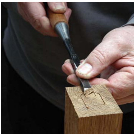
Gooseneck socket is chiselled out in the end grain of the post
