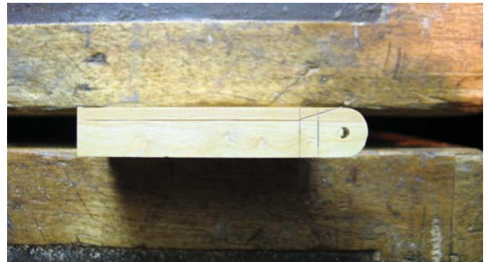
With the pin in place, the spacer was used again to connect the gauge line to the radius, 8mm from the centre of the pin
