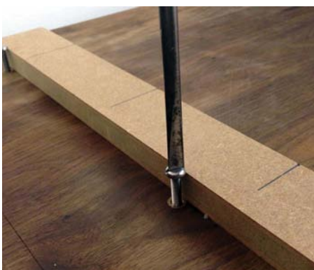
Carry out a dummy run with the screws to expand the brass sleeves in their hole
