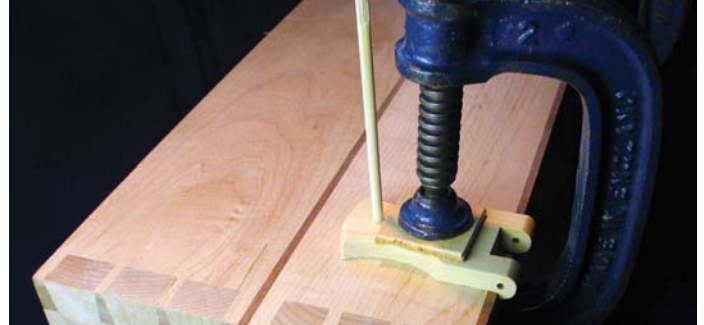
The hinge glued in place, located by the bamboo skewer and the recess in the top
