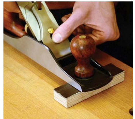
The bench plane placed on a flat surface with the front of the plane resting on a small wooden block
