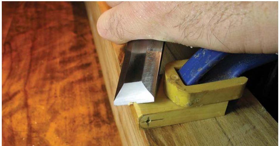
The radius around the pin can be shaped with a chisel and plane ...
