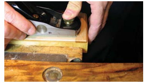
Planes tend to rock about on small pieces making it difficult to achieve a flat surface. This can be overcome with downward pressure on the toe, candle wax on the sole and a very fine setting on the plane
