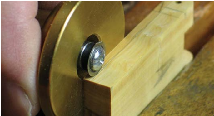
In order to reduce the thickness, a gauge was set to 2.5mm to mark the wood to be removed
