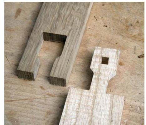
The two mating parts of the pinned gooseneck or 'Komisen-uchi' are marked out and sawn, one used as a template for the other
