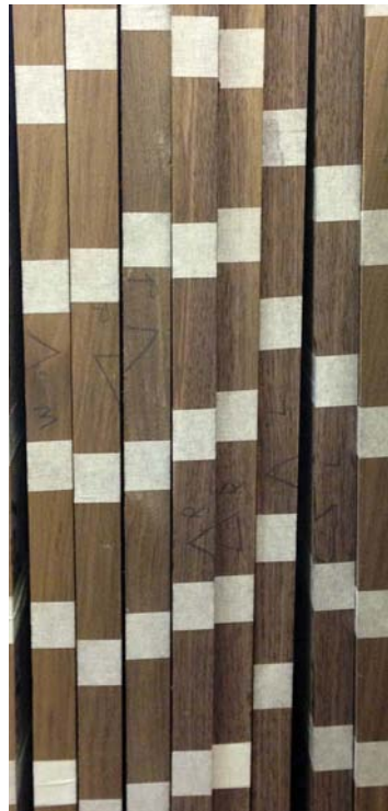
Masking tape is a quick and easy way to fasten lippings in place while the glue dries
