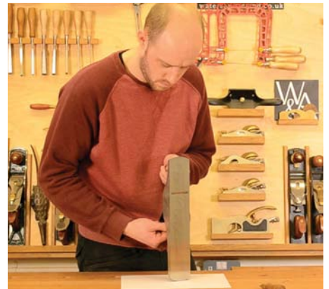
Hold the plane upside down to examine the amount of blade projection
