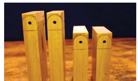
Now ready to be planed to a thickness and length
