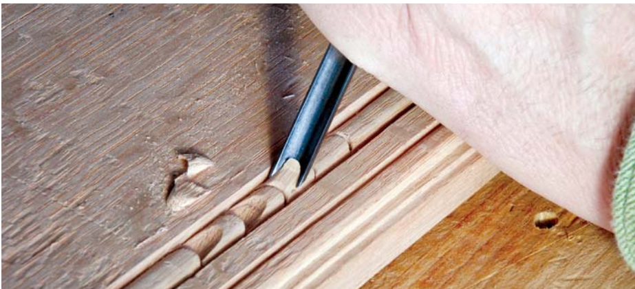
Here is the chip coming up as the gouge meets the first incised vertical cut. Learn this and any blank piece of oak becomes something more
