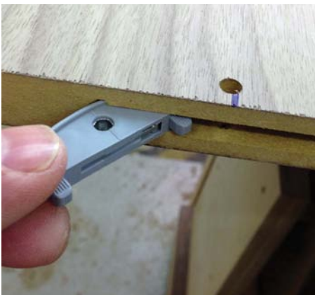
The P2 connectors slide into a slot and are prevented from falling out
