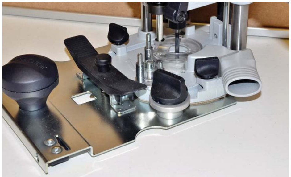
This is ready to use. The large rocker bar releases the locating pin from the guiderail so the jig can slide to the next hole. Bottom left you can see one of two adjustable blocks that remove any play between guide plate and guiderail
