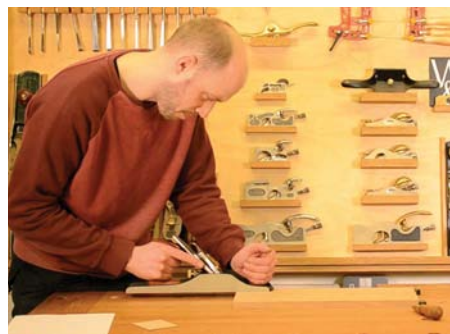
Begin the stroke with more downward pressure through the front knob
