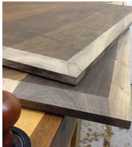
The worktops are finished underneath and brought to their final dimension just prior to fitting
