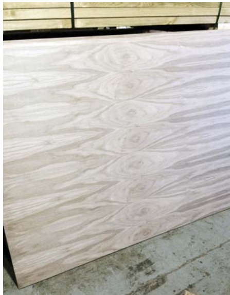
A crown cut veneer face. Hardly likely to be found on a board made of solid timber
