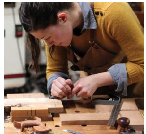
Create a 'V' groove for the saw
