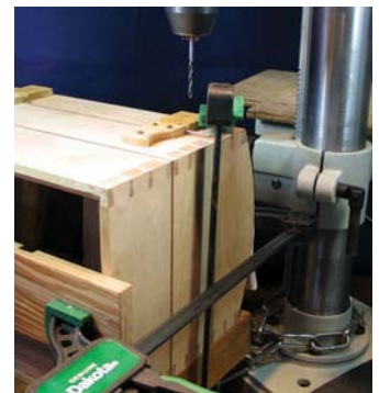
Box with the lid cramped to the bottom, 3mm holes drilled through the hinge and box side for the bamboo skewers. Note the cramp preventing the flap from rising up the drill bit
