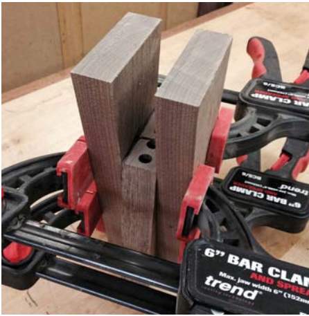
Dowel holes were drilled into the middle section of the feet before gluing up
