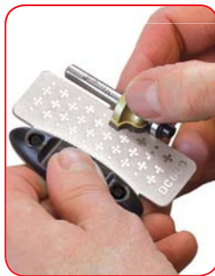
Specialist stone designed for router cutter sharpening.
