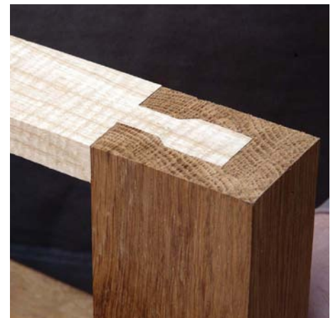
The Kiguchi-ari or gooseneck corner joint is fitted
