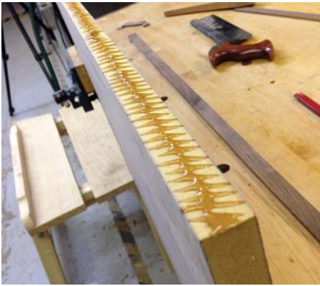
MDF is very porous so apply glue right up to the edge to ensure a good join
