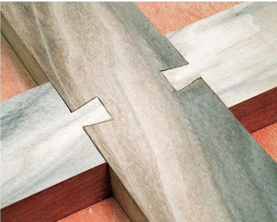
The Shi-ho-ari-kumi-te dovetailed cross lap joint is trial fitted ready for gluing
