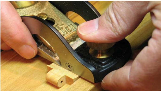
A flat surface restored with a rebate block plane, level with the gauge lines
