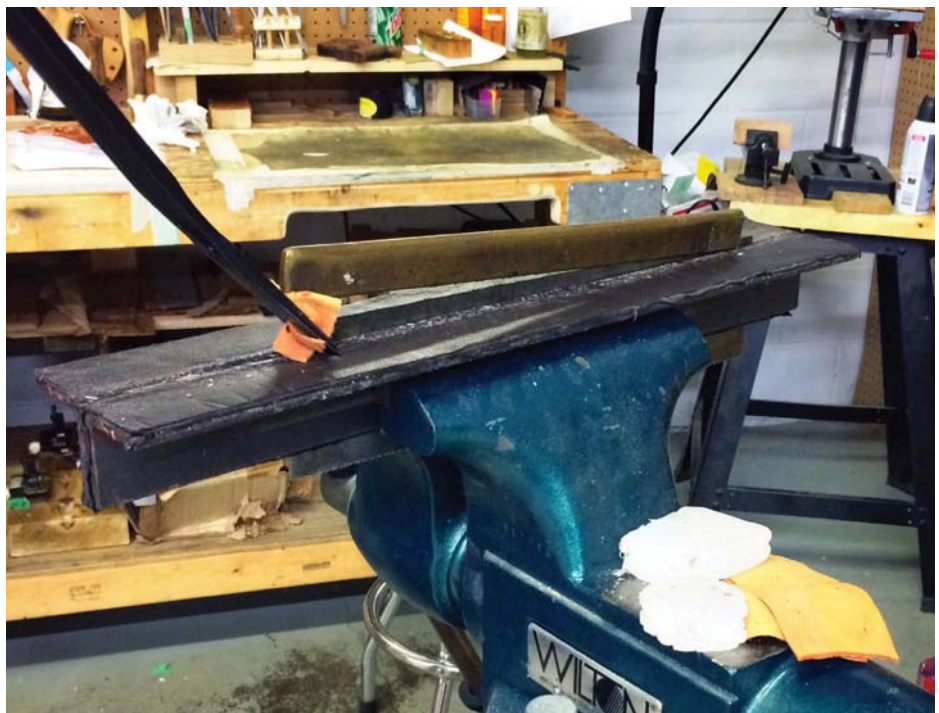
Raising the saw back to separate the handle, back and fasteners
