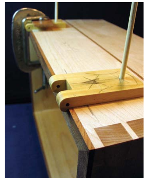
Checked for alignment, cramped, drilled and pegged with a bamboo skewer
