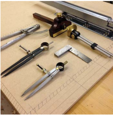
A full-size rod is the best way to locate fixing holes and establish the size of drawer components
