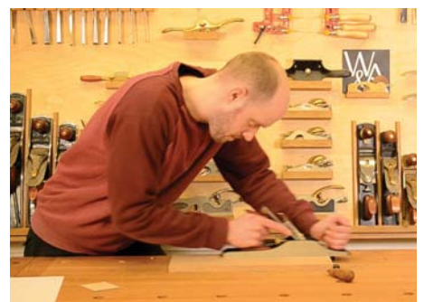
Transfer the balance of pressure to the rear tote as you complete the pass
