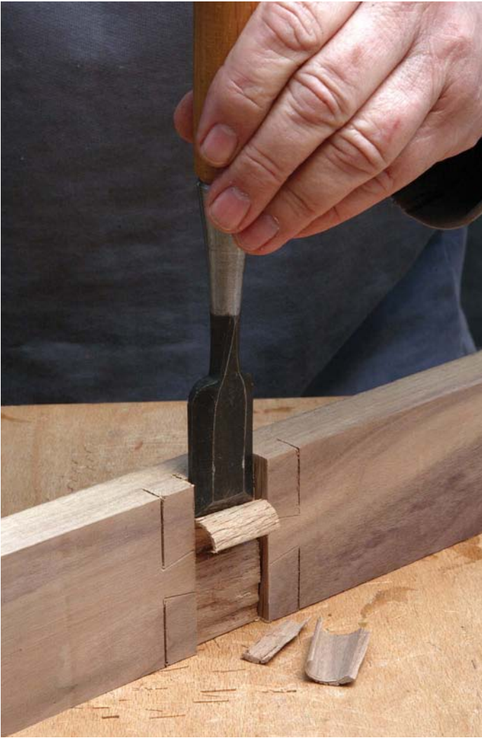
Central channel between the two opposite tail pins is pared out with a wide chisel
