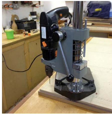
Adjust a portable drill press to drill perpendicularly to the face of the board
