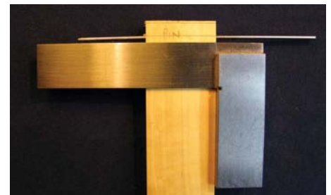
With the pin in the hole, the squareness can be checked
