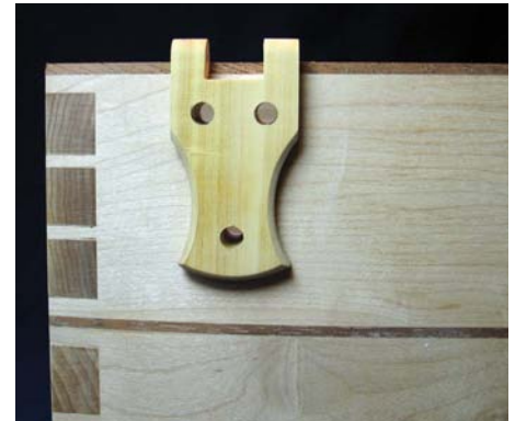
The 5mm holes ready for the pegs
