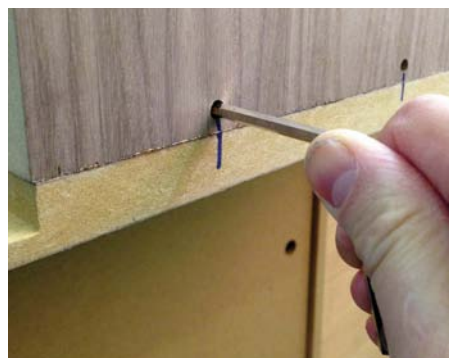
Align the components and lock into place with a hex key
