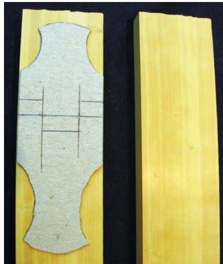
A rough cardboard template used to find the position of the pins
