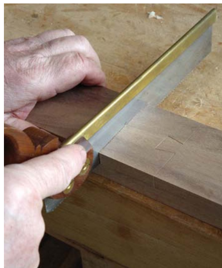
Sawing the central channel between the tails the blade is held level so as to make a horizontal base to the kerf ➤
