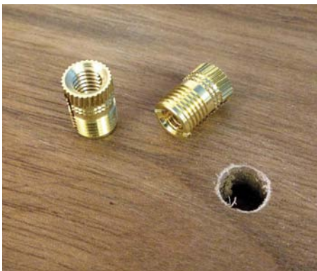
The brass sleeves are a tight push fit. Chamfered tops are easier to locate when it comes to assembly
