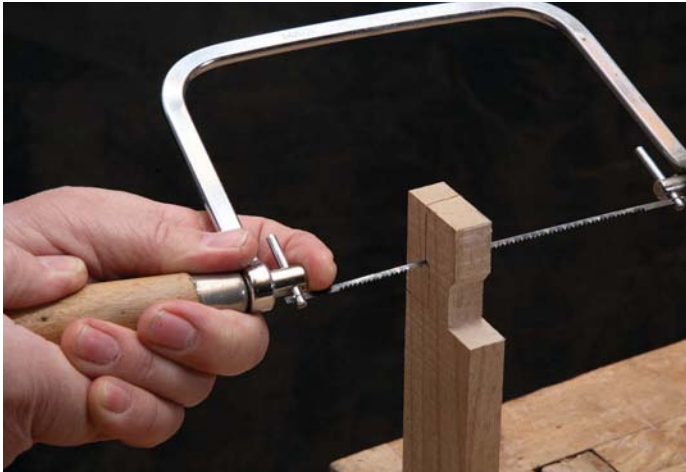
The gooseneck shape for the Kiguchi-ari is marked out in pencil then sawn with a combination of tenon saw and coping saw
