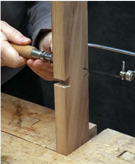
Cutting the full depth sockets for one side of the Shi-ho-ari-kumi-te dovetailed cross lap joint
