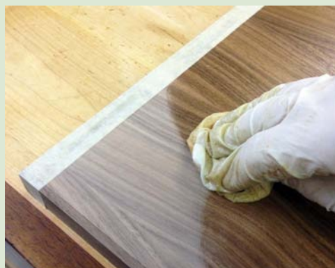
Wetting the surface of the veneer with water to raise the grain
