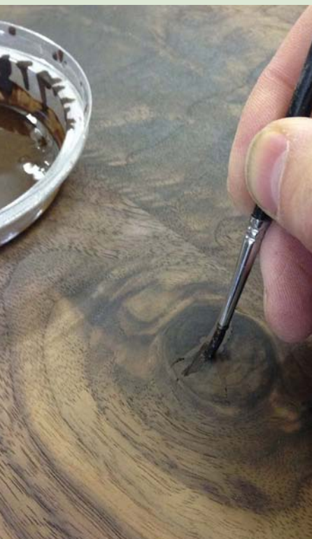
Apply the polish to the filler with a fine brush
