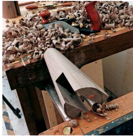
More hand work was required to shape the feet
