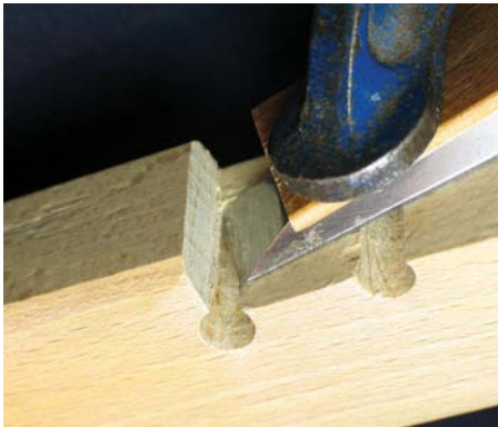
The 'pencil sharpener' type dowel cutter
