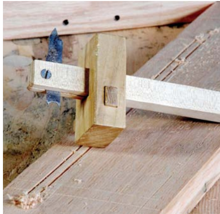
Make your scratch stocks from hardwoods. This one has a maple staff, an ash fence/head and a hickory wedge. A mixed bag to be sure, but it's worth keeping a selection of dry, straight-grained hardwoods around for just this sort of project
