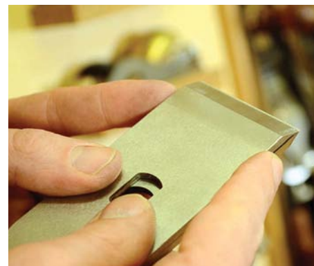
Align the sides of the blade with the chipbreaker
