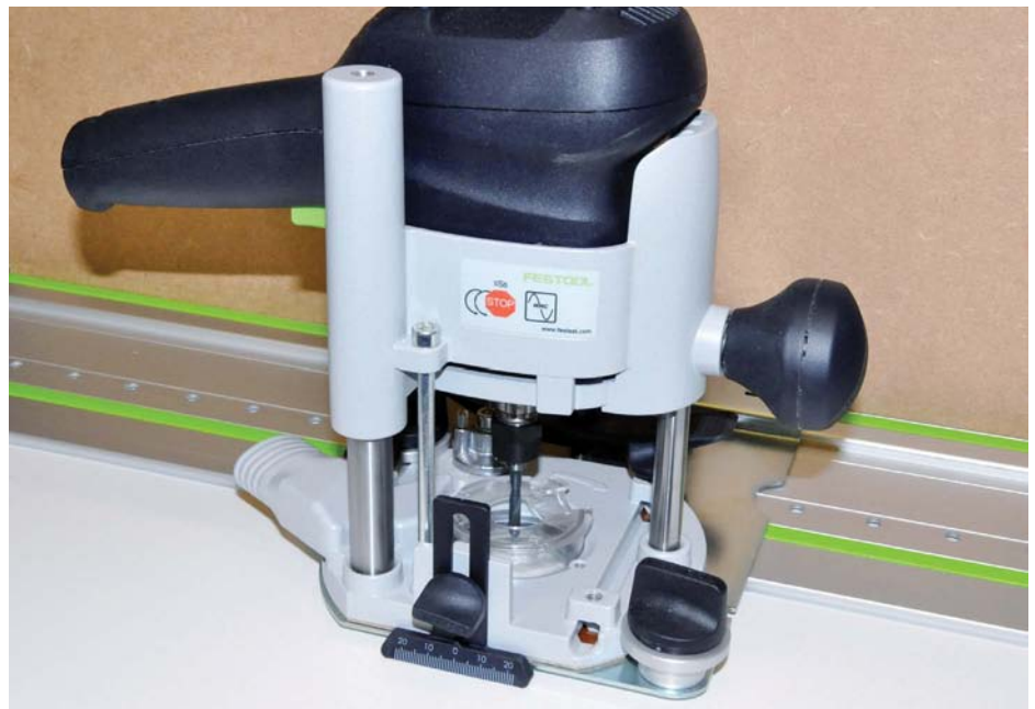
The OF 1010 router snugly in place on the baseplate. One of two clamps can be seen that hold it in position. It is sitting on the special guiderail and you can just see the row of locating holes
