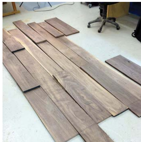
Machined stock is easier to place in sequence and match the ends of boards as they butt up
