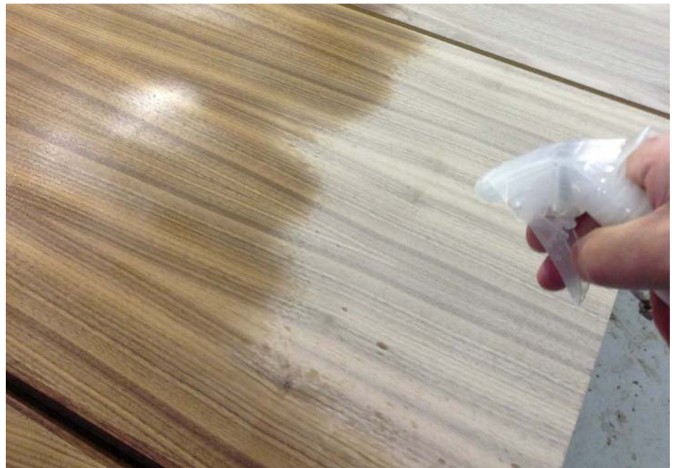
Wetting the surface of the veneer with water to raise the grain
