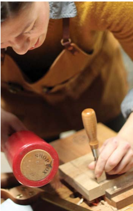
Mark the thickness of the dado using chisel width
