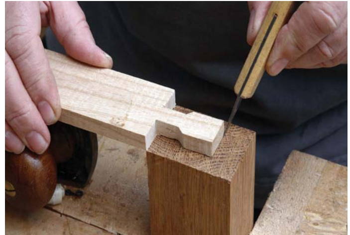
A sawn-out gooseneck pattern is used as a template to mark the socket outline on the end grain of the post
