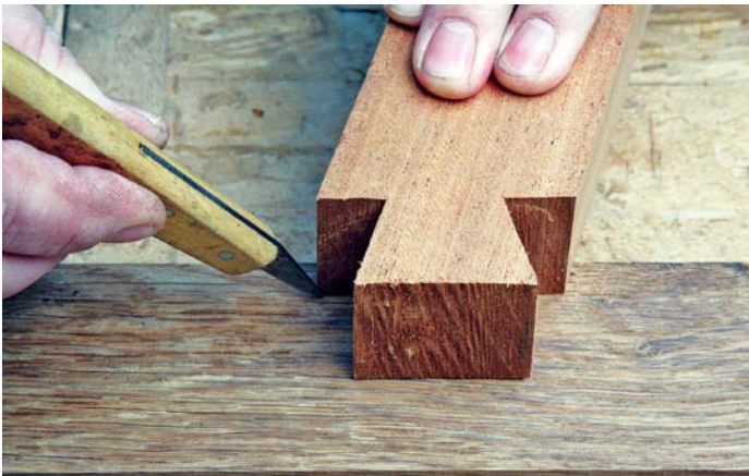
Dovetail shaped pin is sawn to full depth, then used as a template for the socket. In this case, it is angled to make a Hiuchi-ari-otoshi joint
