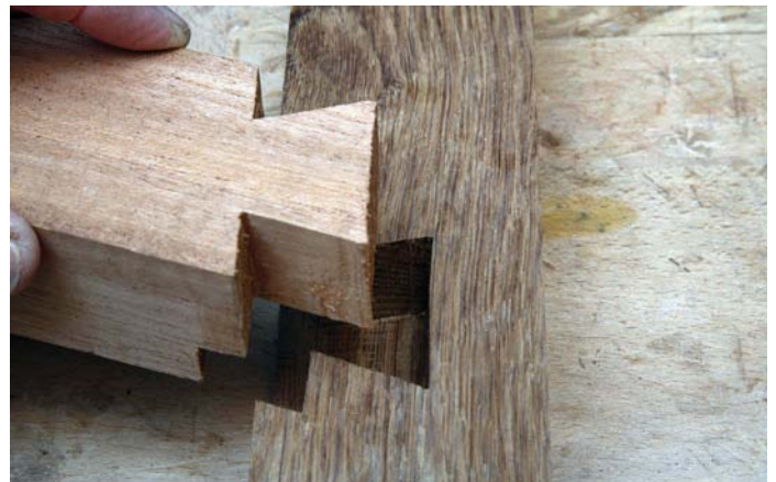
Two halves of the Hiuchi-ari-otoshi are fitted together, leaving the dovetail pattern visible on one side of the joint only
