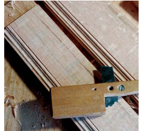
The most common form of scratch stock, this time it's made from an offcut of riven oak. You can cut a shape on each end of the blade, then switch it around for a different moulding. Make these as you need them. The price is right, as is its effectiveness and ease of use
