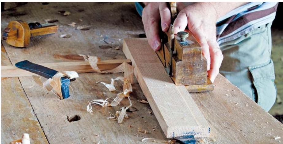
This is a moving fillister plane, which is basically a rabbet plane with a movable fence attached to its sole. The best ones have skewed irons. This one has a depth stop that you needn't be concerned with for this sort of work
