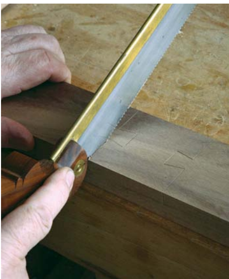
Sawing the shoulders of the dovetail the blade is held at an angle so it will not cut into the tail itself
