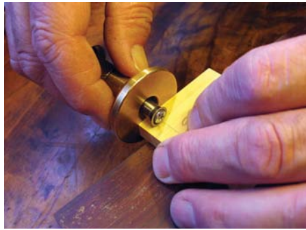
Cutting the segments is similar to cutting dovetails, they can be marked with either a gauge or square
